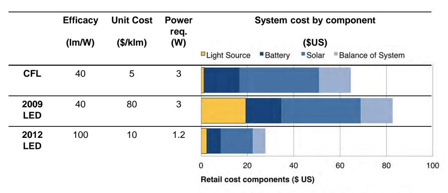
Assumptions: 120 lumens for 4 hours each day, solar cost \$5/W, solar resource 5 kWh/m2, battery cost \$0.3/ Wh, BOS cost \$2/W, 70% derating
