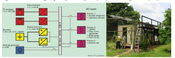
Figure XI. Existing hospital hybrid PV system (3kW) with diesel generator (9kW) as backup
